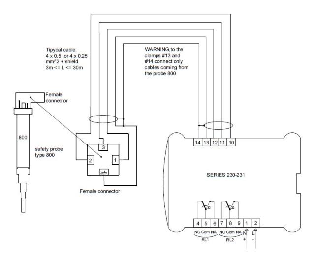
5.3 - Electric power supply for 230V-AC version (terminal: 1=Neutral; 2=line)
