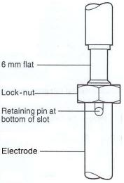
5. Holding the assembly firmly, insert the retaining pin until its protrusions from both sides of the electrode are symmetrical.
