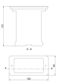
The level switch can be installed on the panel door of the cabinet, using the provided accessory kit, which includes a rubber gasket, a frame and 2 fixing crews. It is provided also a plastic clip, in order to possibly use the mounting DIN rail.
