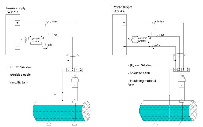
5.5 - Wiring diagram (two wires) for 450 with user not galvanically isolated
