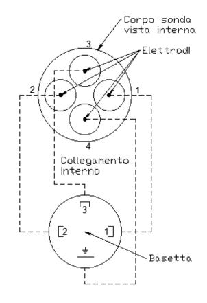
The above drawing indicates the top view of the electrode holder with the lid unscrewed and of the male DIN connector on the electrode holder. The electrode holder does not have a ground connection, which, in the case of a metal tank, is still secured using the threaded body of the electrode holder.
