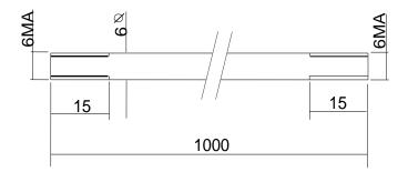
This electrode has the purpose to extend the conductive end of the electrode holder, obtaining different levels for common, minimum and maximum. It is possible to join several modules, 1 meter long.
