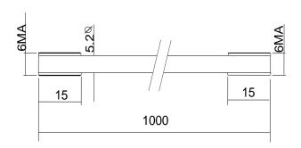
This electrode has the purpose to extend the conductive end of the electrode holder, obtaining different levels for common, minimum and maximum. It is possible to join several modules, 1 meter long.
