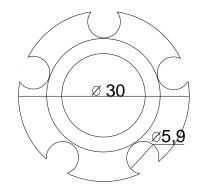
This spacer has the purpose to keep spaced the 6 mm diameter electrodes, when their length may cause a contact between them or with the tank.
